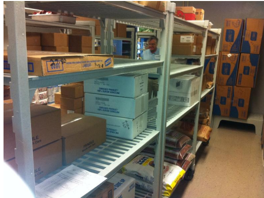
Kitchen shelving should have wire racks and lockable wheels.
